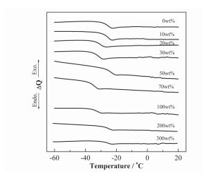
Fig. 6 DSC profiles of polyether/NZSP composite electrolyte composite solid electrolyte.
