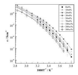
Fig. 7 Temperature dependence on ionic conductivity for polyether/NZSP composite electrolyte composite solid electrolyte.
