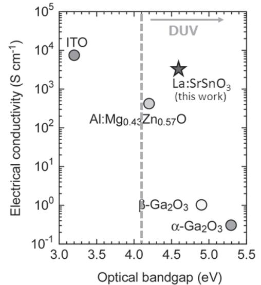
Figure 1 – Optoelectronic properties of transparent semiconductors and the results obtained from this work.
