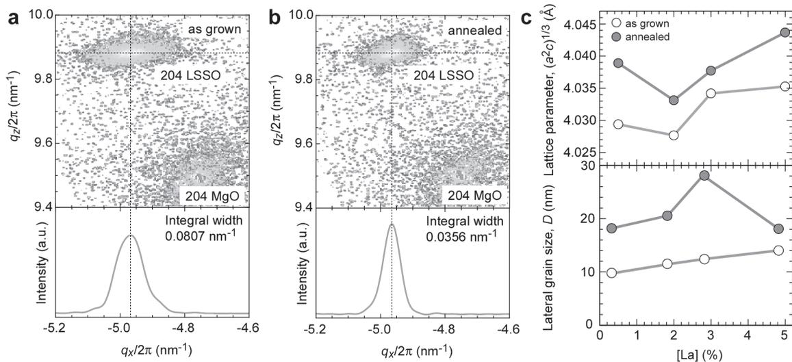
Figure 2 – (a, b) RSMs around 204 LSSO diffraction spot of (a) as grown and (b) vacuum annealed films. The cross-sectional diffraction patterns along  $q_x/2\pi$  direction are shown at the bottom of each RSM. (c) Changes in (top) the average lattice parameter and (bottom) lateral grain size of the as-deposited LSSO films (white) and annealed LSSO films (red) as a function of La concentration.
