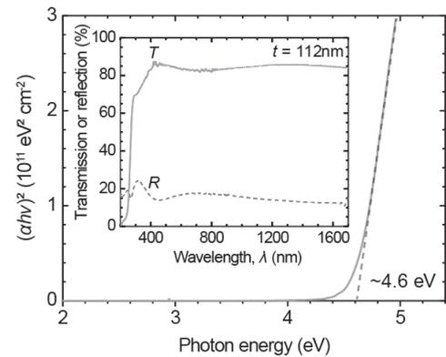
Figure 5 – Optical properties of vacuum annealed 3% LSSO film. The  $E_g$  was  $\sim 4.6$  eV, which can transmit DUV lights.
