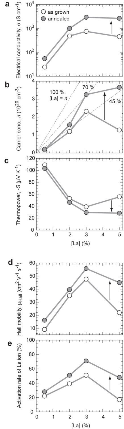
Figure 4 – Electron transport properties of the LSSO films as a function of La content (%). (a)  $\sigma$ , (b)  $n$ , (c)  $-S$ , (d)  $\mu_{\text{Hall}}$  and (e) Activation rate of La dopants.
