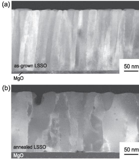
Figure 3 – Cross-sectional LAADF-STEM micrographs of (a) as-grown and (b) vacuum annealed LSSO films.
